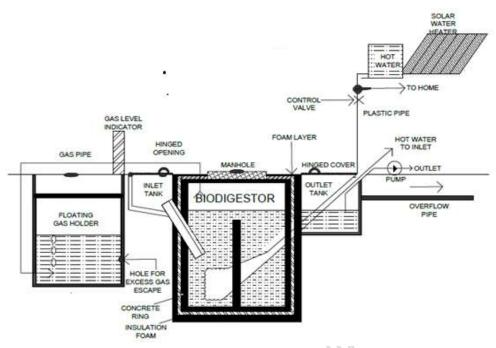
Figure 1. Improved floating dome biogas digester (named as Udupi Krishna-Manipal or UKM model)
