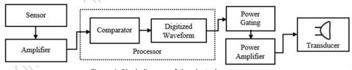
Figure 1. Block diagram of the electrolarynx
