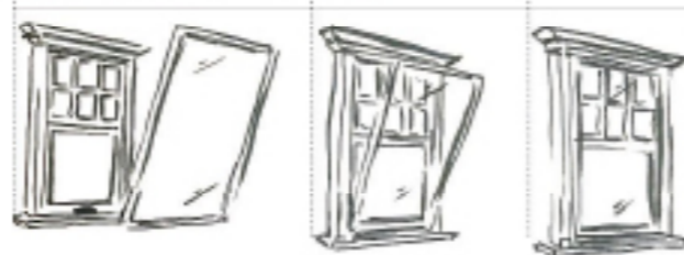
INSTALLATION OF WINDOW INSERT
