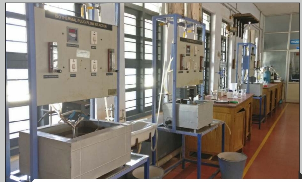
Chemical Reaction Engineering (PFR & CSTR setups)
