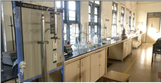
Mass Transfer Lab- Packed Bed Distillation Column
