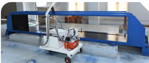
Prestressing Rig and Hydraulic Jack
