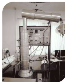
Pilot Plant Batch Distillation Column
