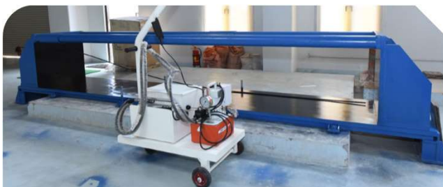
Prestressing Rig and Hydraulic Jack
