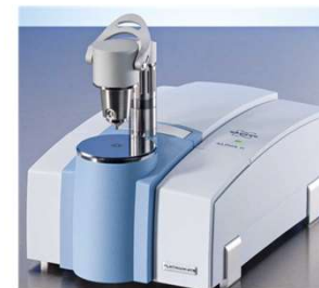
FTIR: ATR and transmission mode
